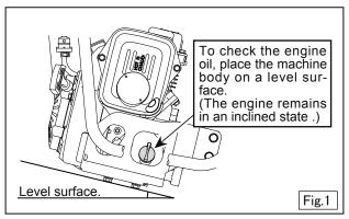
Place the machine body on a level surface and look at the oil gauge on the protective sleeve, from the right side. See if the oil is at the specified level. (Fig.2)
