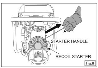
5. After the engine has started, open the choke lever gradually until it is wide open. Pay attention to the sound of the engine to guide you in the amount to open the choke. After the engine has started, be sure to warm up the engine at low speed for 3 to 5 minutes. During this time, check the machine for leaking fuel, abnormal sounds, or abnormal exhaust color or odor.
