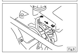
2. After operation is started, adjust the throttle lever a little until the rammer tamps the soil correctly. When the engine is running within the specified rpm range, the rammer will be the most effective. If the engine runs too fast, the tamping force will not be increased. Instead, the spring resonance will decrease the tamping force and damage the machine.
