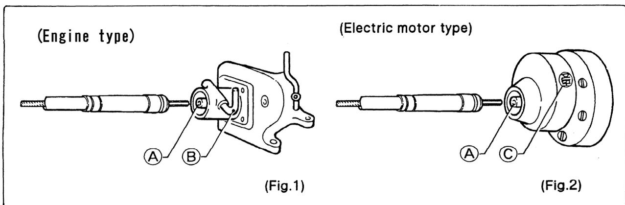
2-3 To connect Flexible shaft set to prime mover, insert Hexagonal joint to the socket (A) and then pushing the Shaft coupling until locked by turning the lever (B) or by pushing the push button (C), if necessary.
